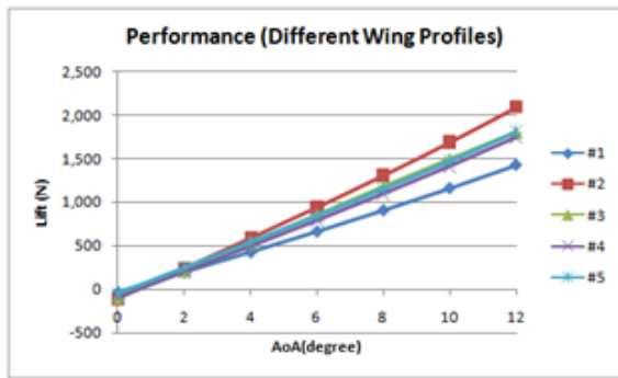
Figure 13: Lift Performance with different wing profile.
